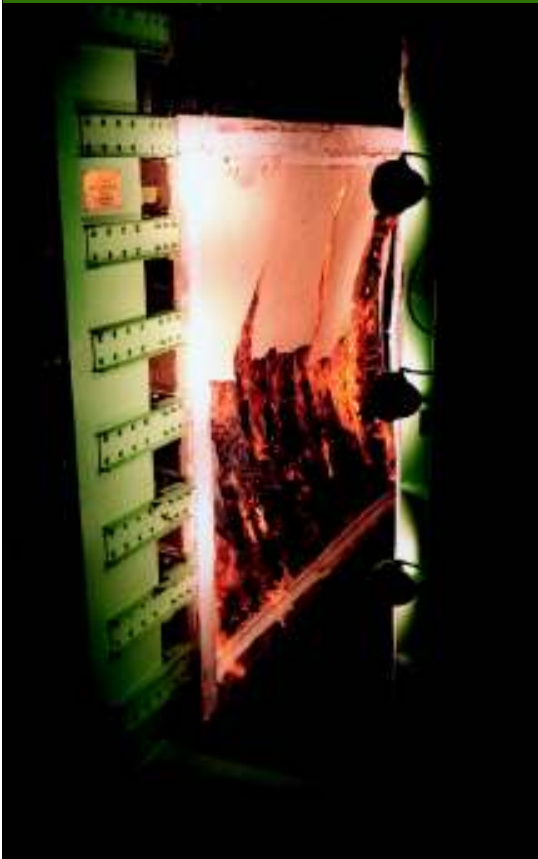
FIGURE 2: Wood-Stud Wall Assembly After 1-Hour Test
