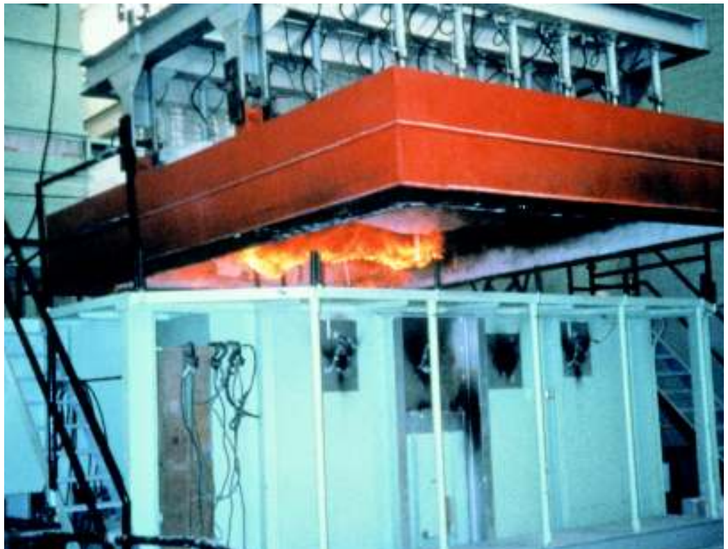
PHOTO 4: Wood construction assembly being tested in the fire chamber at the National Research Council of Canada.
