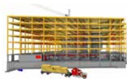
Figure 6.6: 4D sequencing with Navisworks for T3, T3, Minneapolis, MN. (Image courtesy of StructureCraft Builders Inc.)
