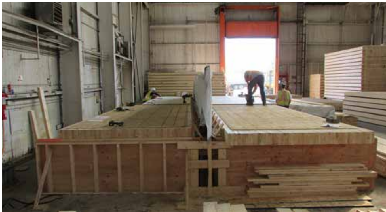
Figure 6.3: NLT fabrication set-up. (Photo courtesy of StructureCraft Builders Inc.)
