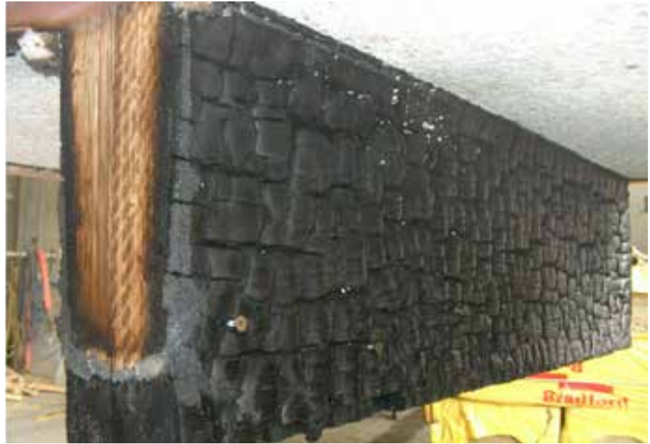
Figure 3.4: Representative Example of Effective Depth. Photo adapted from the CLT Handbook [3]
