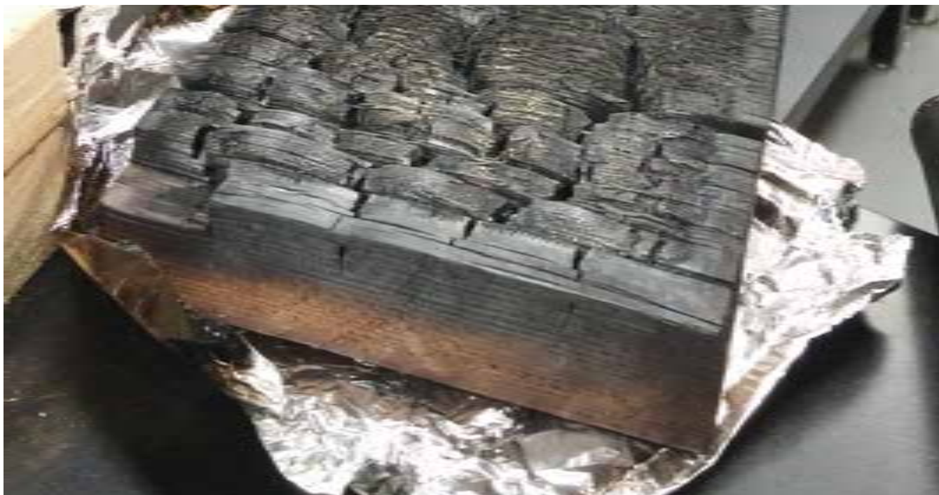
Figure 3.3: Wood Charring. (Photo courtesy of Holmes Fire)
