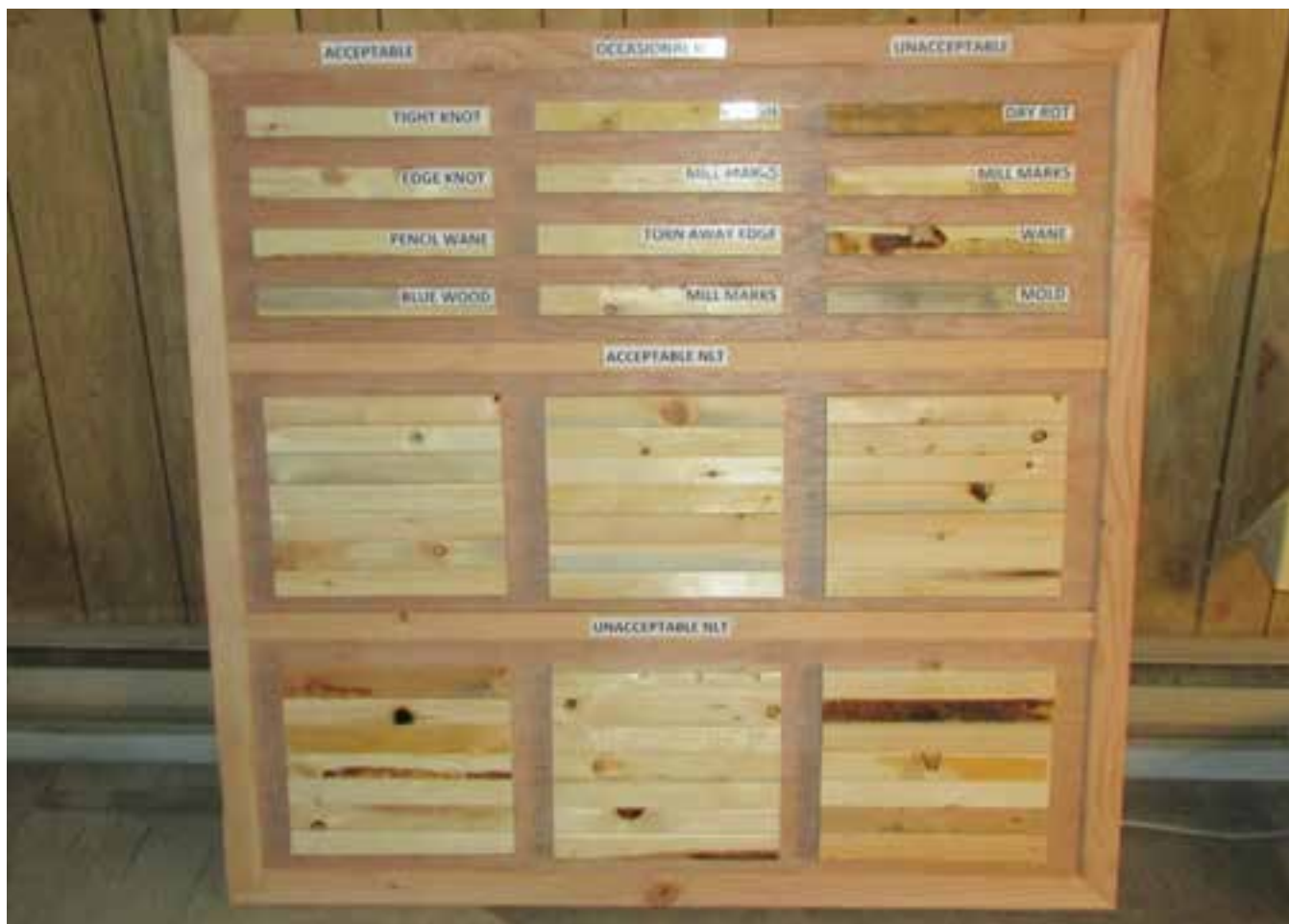
Figure 6.2: Example of aesthetic grade boards for NLT panels. (Photo Courtesy of StructureCraft Builders Inc.)
