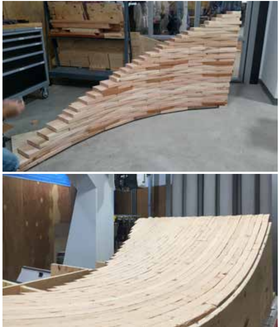
Figure 2.8: CNC milled compound curve prototype. (Photo courtesy of Perkins+Will)
